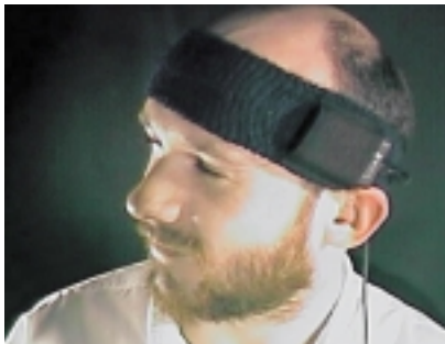
A computer mouse operated by head movement
